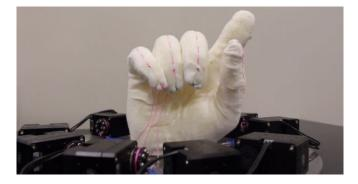
Fig. 1. A soft robotic hand with naive tendon routing. A more clever actuation layout could have likely achieved this pose with fewer tendons
