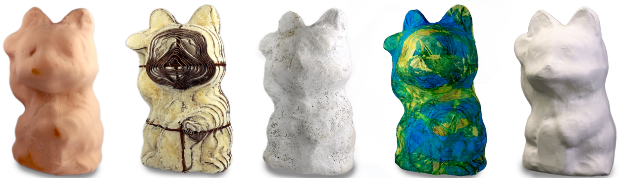
Figure 22: Different possible applications of packable springs. From left to right we used plastic clay, construction foam, gypsum, wallpaper and clay to cover or fill the shape.
